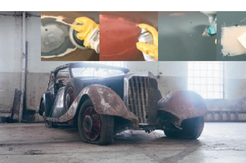
Standox recommends a two-coat build-up consisting of an acid primer and a 2K filler. The acid primer has a passivating and corrosion-inhibiting effect. In combination with the 2K filler, it also provides excellent adhesion to the metallic substrate on the one hand and to the topcoat on the other hand. The 2K filler isolates sanding marks and pores and helps to even out the surface. It is the ideal basis for the topcoat.
