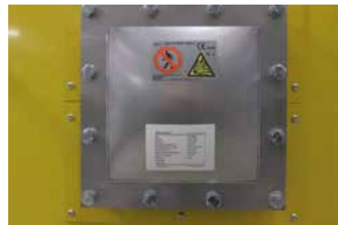
Optional: ATEX blast cover offers an exit for explosion, preventing total machine destruction.
