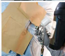
Apply filler. Mask and apply Standox 2K Filler.
