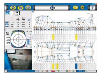
Just press the bull's-eye shaped button for automatic measuring. The ASP function displays photos of the measuring points automatically on-screen as the Measuring Slide moves from point to point.
