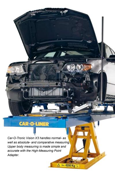
The Measuring Slide's five sophisticated sensors provide real-time data three times per second.
