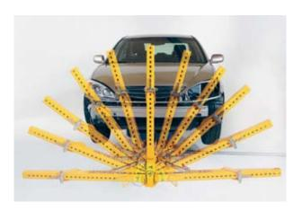
3. The draw aligner can be adjusted to any position. It is self-locking and easy to mount in the right spot.
