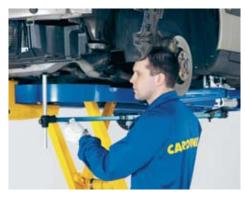
SPEED Check is a device for quick and easy comparative measuring.
